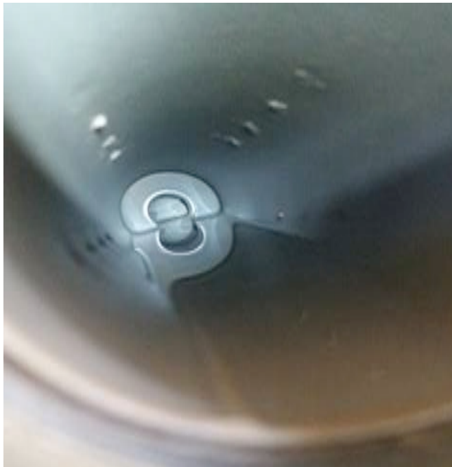
Figure 3: Image of inside of 304 stainless steel pipe after magnetic treatment. Accumulations of loosely bound calcium precipitates are clearly seen near the location of the magnetic pole faces of the Hydrodyne magnetic treatment bracelets.
